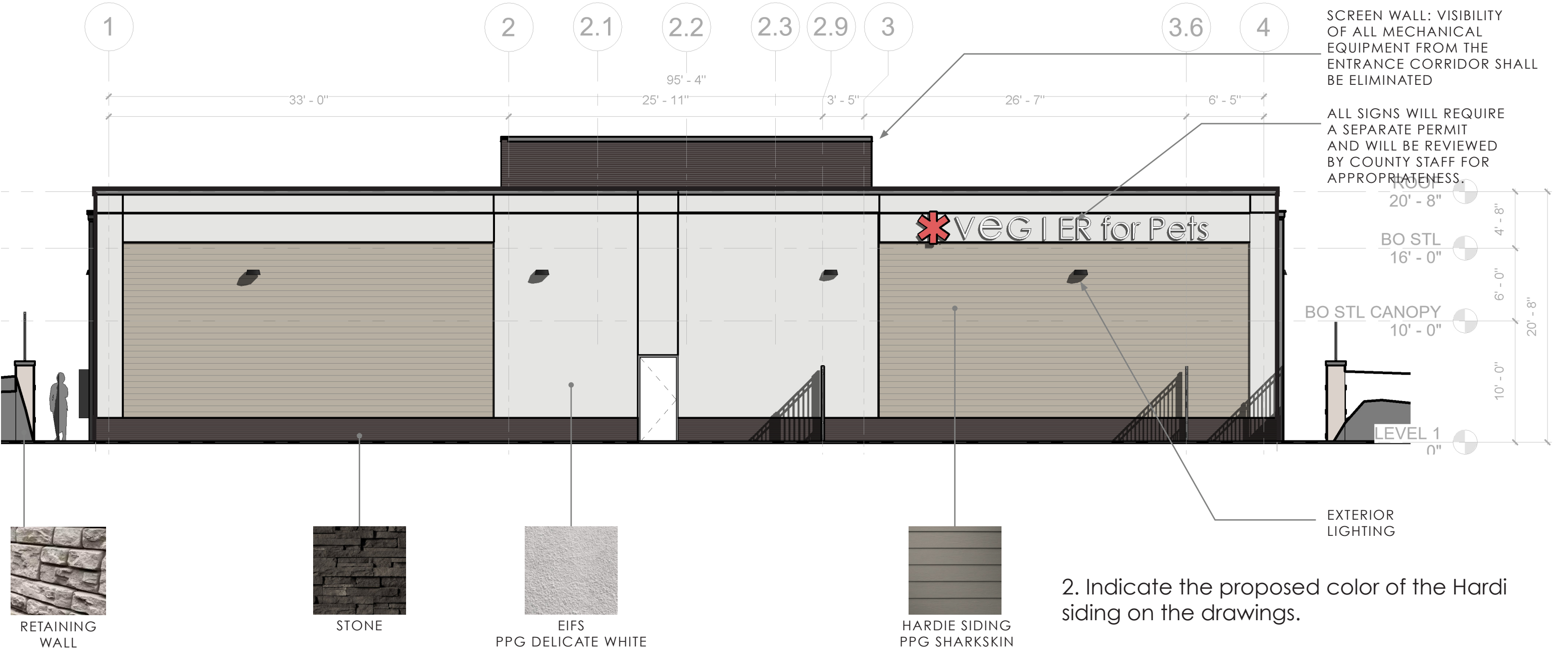
SOUTH ELEVATION - ALONG HYDRAULIC ROAD
